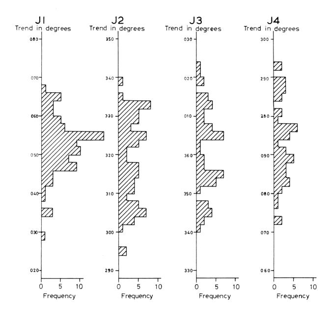
Text-fig. 3. Histograms showing the variation within each of the joint sets.
